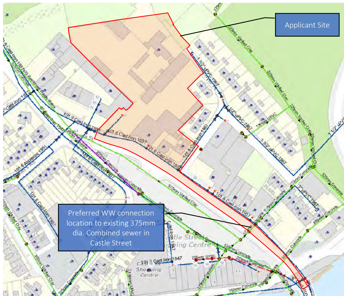
Figure 6-2 Preferred Wastewater Discharge Point
