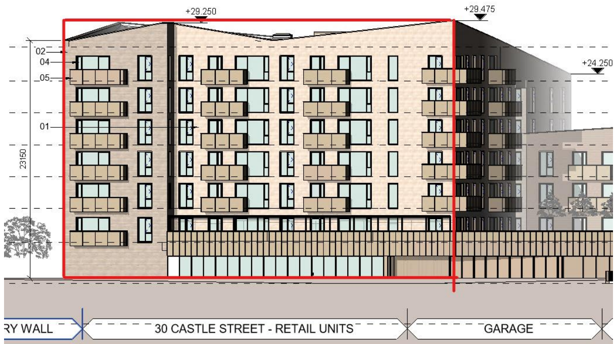
FIGURE 11. TYPICAL ELEVATION FOR WHICH THE RATIO OF GLAZING TO SOLID WALL WAS CALCULATED. IN THIS INSTANCE, THE PERCENTAGE OF GLAZING WAS CALCULATED AT 26.9%.
