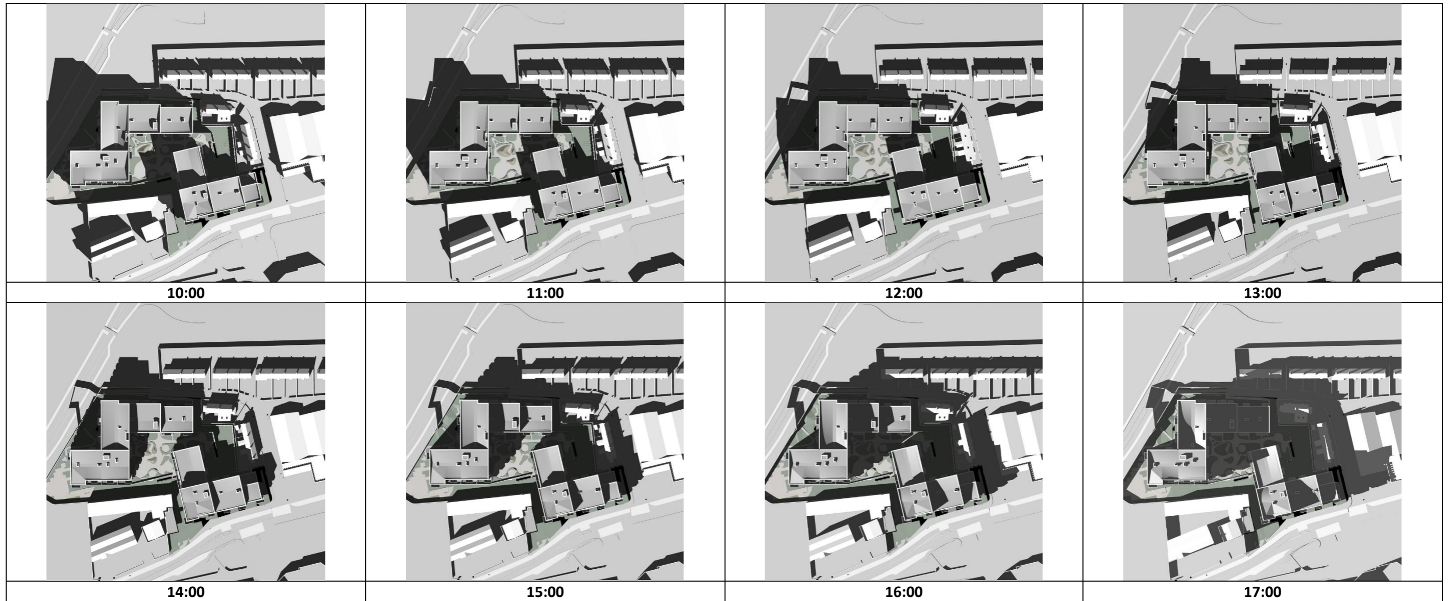
Fig B1: Sunlight and Site Shading Diagrams - Equinox (March 21st): 08:00-17:00 hrs
