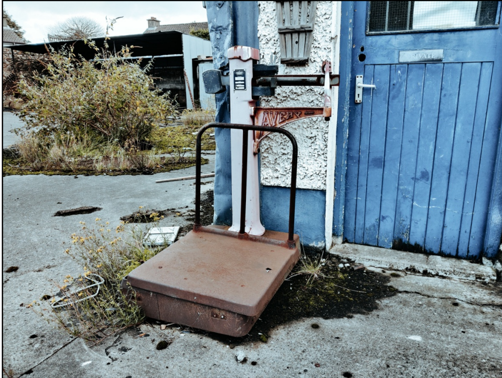
Plate 15 Avery platform weighing scales, type 3205 ABA, manufactured Birmingham, England (1950-1970).
